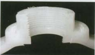
Spin welded inserts require adequate space of the chuck.
