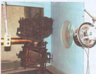
Molds are biaxially rotated in an open oven to melt the resin.
