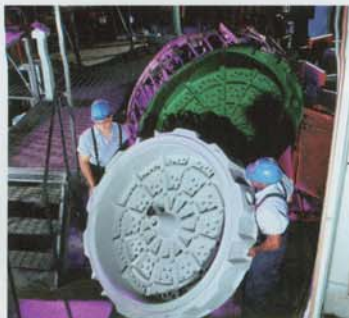
This large rotationally molded water filter section measures 6 feet across.
