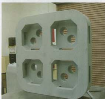
Features such as these add a great deal of rigidity to a part.
