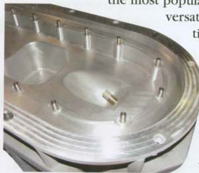
Machined rotational molds are the most accurate and expensive.
