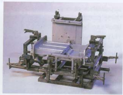
Cast aluminum molds are the most popular method of making rotational molds,
