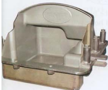
Sheet metal molds are a very cost effective alternative for rotational molds.
