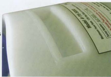
Parting lines can sometimes produce thick witness lines as shown in this photo.
