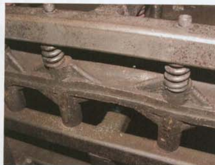
Compression springs are used between the frame and casting to absorb tolerance variations.
