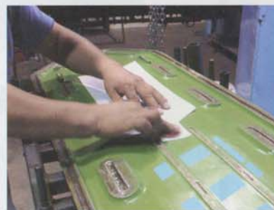
Transfer graphics are applied to the mold surface before the mold is filled with resin
