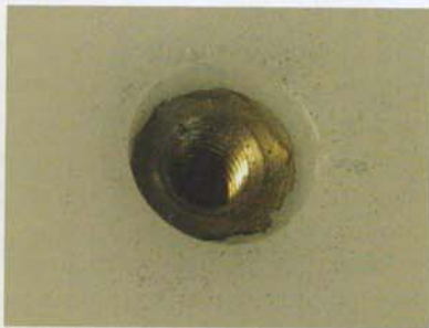
Molded in inserts are placed in the mold before the resin is loaded.
