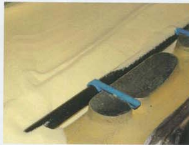
Granular resin has a low bulk density occupying more volume than molded resin.
