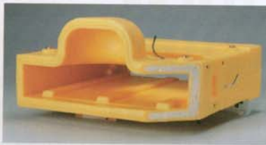
Polyurethane foams add rigidity and insulation to parts.
